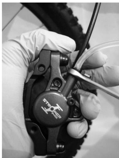
**6** Turn the spanner to open the bleed nipple (anti-clockwise quarter turn). Begin to inject fluid from the calliper syringe. You will start to see fluid emerging from the brake lever into the tubing with any air bubbles which were previously in the brake system.
