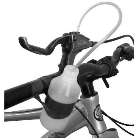
**NOTE:** If you leave your wheel and pads in situ, wrap a cloth around your calliper to protect your disc and pads from fluid spillages.
